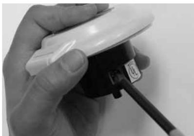
4. Back off terminal screws on the rear housing of the inlet. Insert wires into color coded openings on the back of the inlet. Tighten terminal screws to 14-20 in.-lbs. torque. **Make certain there is no wire insulation under any terminal.**
