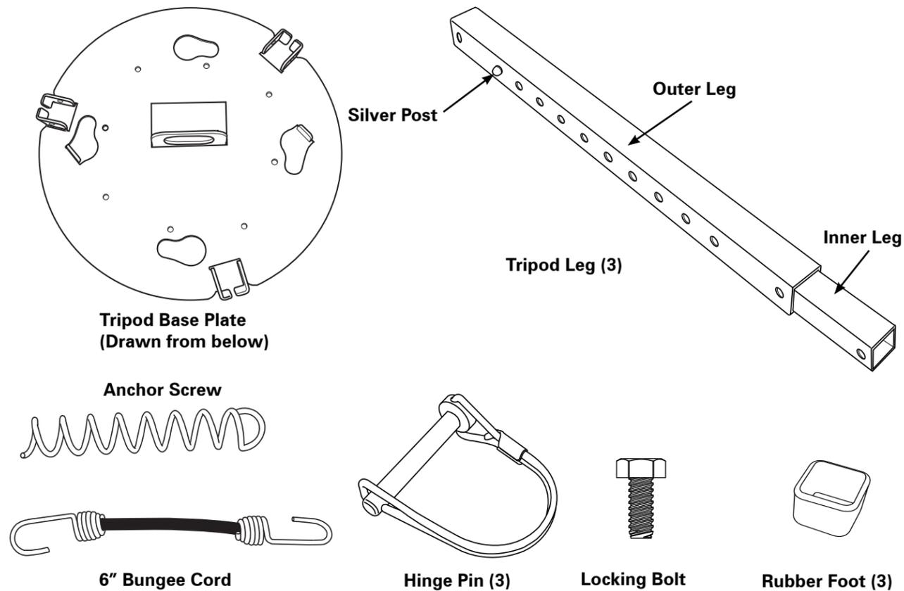
**CAUTION** The Carryout Tripod is designed only for use with portable satellite TV systems. The tripod has a maximum supported weight of 15 lbs. **DO NOT** use the tripod as a step or a seat.
