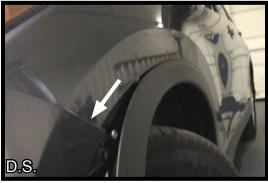
6. Pull the fascia up and outward to loosen from the wheel wells. Apply slight pressure as this does not pull away easily.
