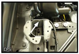
13. Using a chisel, remove the nut in order to slide the baseplate in.
