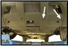
4. Remove the four (4) push pins that are located under the vehicle. There are two (2) on the passenger's side and two (2) on the driver's side.
