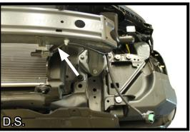
10. On the passenger side, remove the screw on the bottom, outer edge of the bumper core. On the driver side, the temperature sensor will need to be temporarily removed by releasing the push pins. It will be relocated once the baseplate installation is complete.
