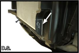
11. On the passenger side, cut straight down to remove the bottom portion. On the driver side, notch up 2-1/2" and straight out.
