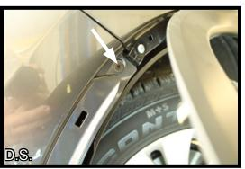
5. Carefully pry the wheel well trim back slightly. With a Phillips screwdriver remove the one (1) screw that is located towards the top portion of the wheel well.
