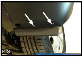
2. Remove the one (1) screw and one (1) push pin that are on the under side of the vehicle, right ahead of the front tire.
