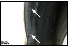
1. Using a Phillips screwdriver remove the screw at the bottom of the wheel well area. There are two (2) push pins that will need to be removed in this area also. Both are located above the screw.
