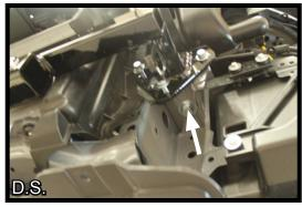
18. Insert a 1/2"-13 x 1-1/2" bolt, 1/2" lock washer and 1/2" flat washer into the bottom side hole. This hole may need to be reamed out slightly. Use a 1/2"-13 nut plate to fasten securely.
