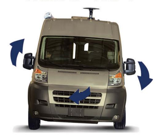
As your motorhome goes around corners the high center of gravity pushes against the side of the RV. As the bottom is clearly planted on the ground it doesn't have much room to move, but the top of the RV is not secured horizontally, so the top continues to move as the bottom stays in place.
