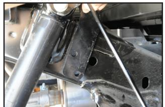
10. Slide front frame brackets to outside of frame and mount front bed rail while keeping frame bracket tight to frame. Tighten all bed rail bolts according to chart on front page.
