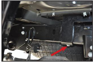
9. Slide rear brackets in to place as shown and bolt using 1/2" x 6" bolt, flat washer, and lock washer. Leave bolts loose. Mount rear bed rail to bracket as shown in bed rail instructions.
