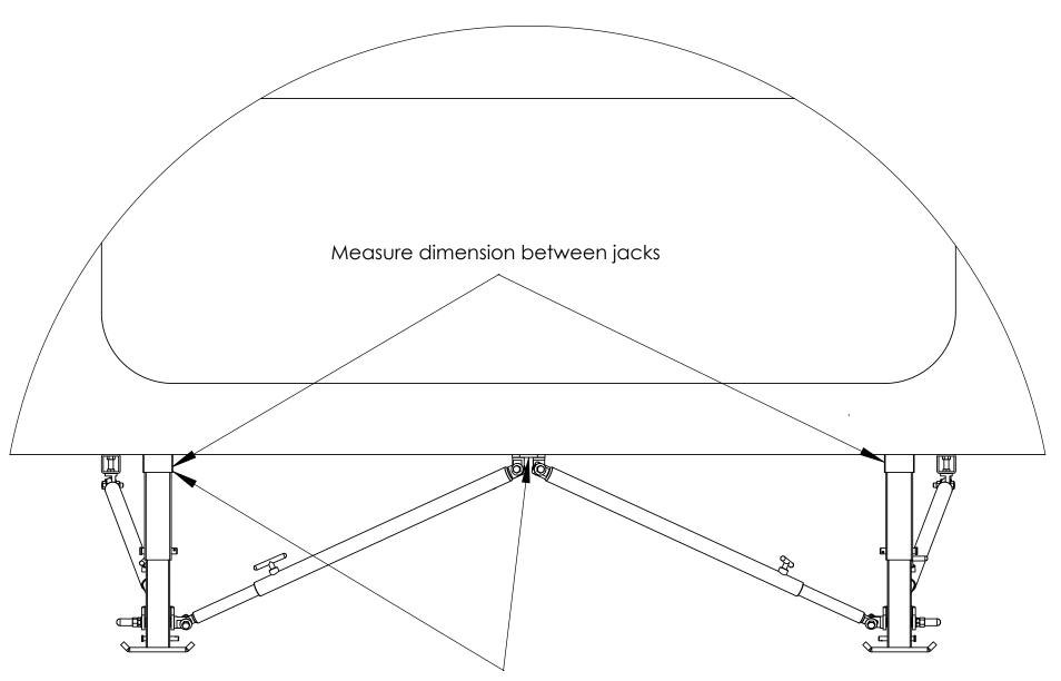
If dimension between jacks is 58" to 66" this measurement should be 1/2 the distance. Example(58" = 29")
