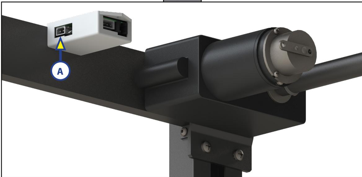
2. Release the brake by moving the release level to the "OFF" position (Fig. 24A).
