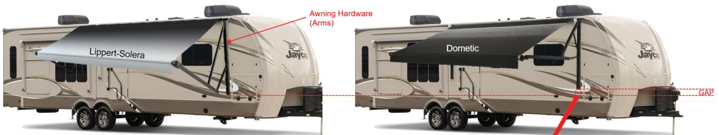
Lippert awning arms are longer than Dometic's. Direct replacement of a Lippert awning with Dometic's leaves a gap. The new product solves this problem by providing a decorative awning arm extension to cover the holes.
