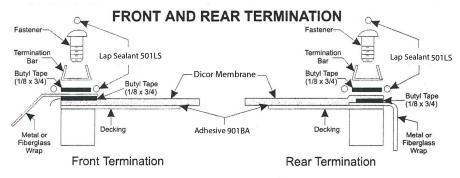
NOTE: Butyl tape should also be used under the membrane where it comes in contact with the unit body at the front, rear, and side terminations. See all termination drawings for correct butyl placement.
