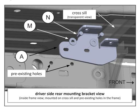
6. Drill five 1/16" pilot holes through the bed, and cross sill where applicable, required for locating the position
