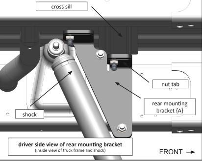
8. Remove the Rear Mounting Brackets and drill out the five (including center base rail hole) rear mounting bracket pilot holes with a 9/16" drill bit.
