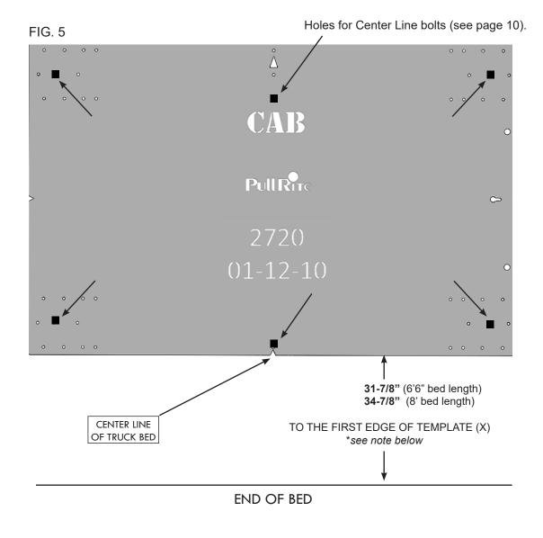
\*NOTE: To insure accuracy of bed holes, follow all steps on pages 8-9 before drilling into the truck
