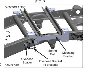
NOTE: Use a hand wrench to tighten the flange nut onto the bolts. DO NOT use an impact wrench, this can easily strip the connection.
