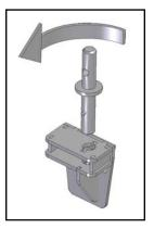
**NOTE:** Vehicles using plastic bed liners may require taller mounting posts (part# 311512) to seat properly into the post holders.
