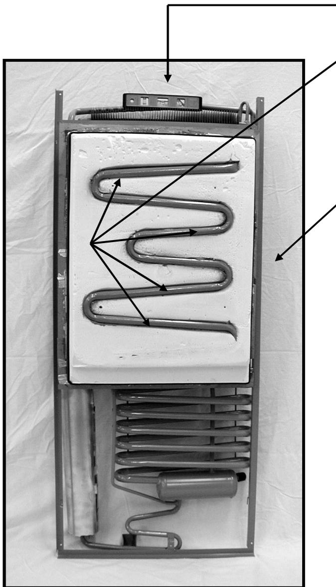
\_\_\_\_\_ Make sure condenser fins at the top of the refrigerator in the back are **level**.
