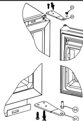
2. Change the position of the cabinet hinges and the strike plate and remove the control housing.
