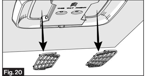
3. The filter can be washed with warm soapy water. Care must be taken to avoid ripping the fabric.
