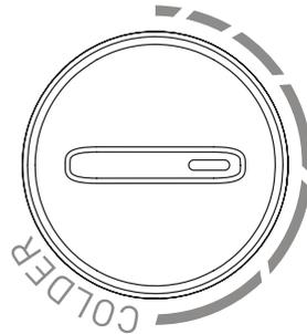
1. Rotate the operating mode control knob to the cool position.
