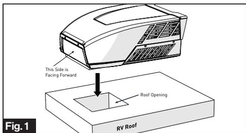
This completes the outside installation of the rooftop unit. Minor adjustments can be done from inside of the RV if required.
