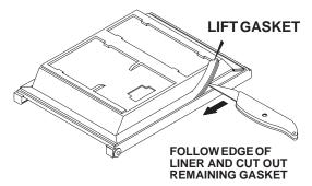
**NOTE: DO NOT** pull gasket from door as damage to plastic liner can occur.
