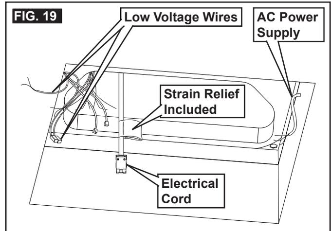
4. Remove the strain relief from its packaging and set aside momentarily.
