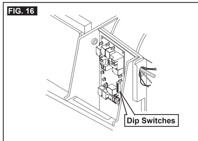
**i** Dip switches are in the "OFF" position when shipped from the factory except heat pump and factory installed heat strip models. On these models the appropriate dip switch, heat pump or heat strip, is in the "ON" position from the factory.
