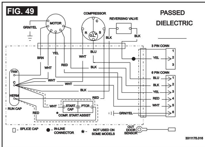
3. 459196 & B59196 Unit Wiring Diagram
