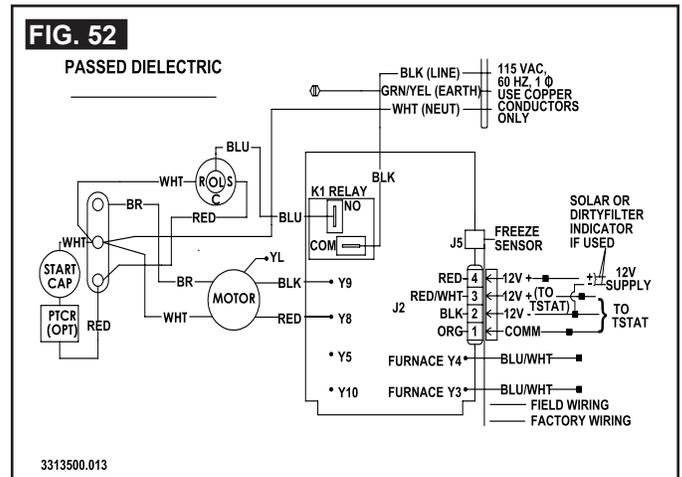
6. 551816, 651815, & 651816 Unit Wiring Diagram
