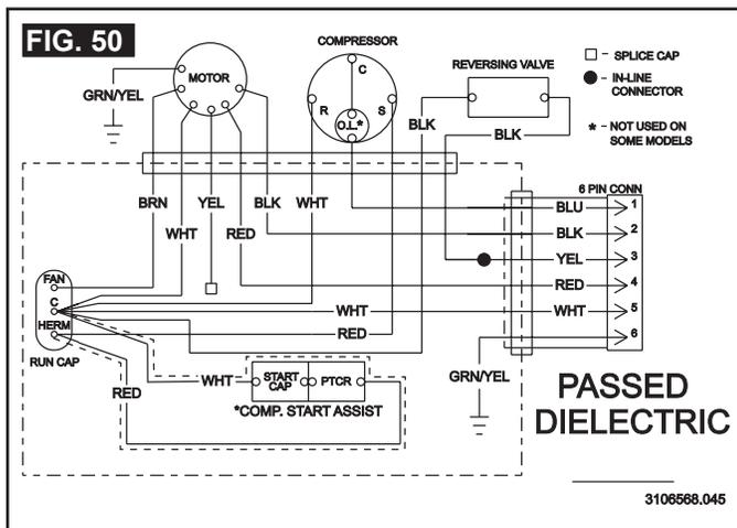
4. 540315 & 540316 Unit Wiring Diagram
