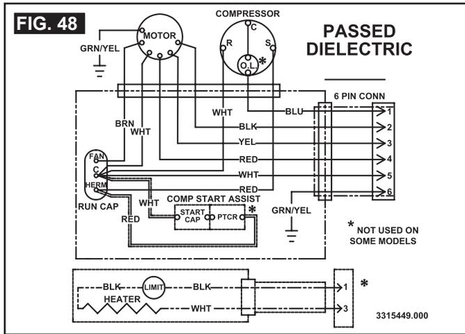
2. 459186 & B59186 Unit Wiring Diagram
