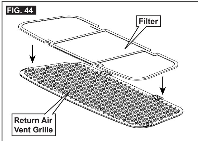
6. Install return air vent grille into the ADB. Slide return air vent grille tab into slot in ADB and rotate up and snap in place. See (FIG. 45).
