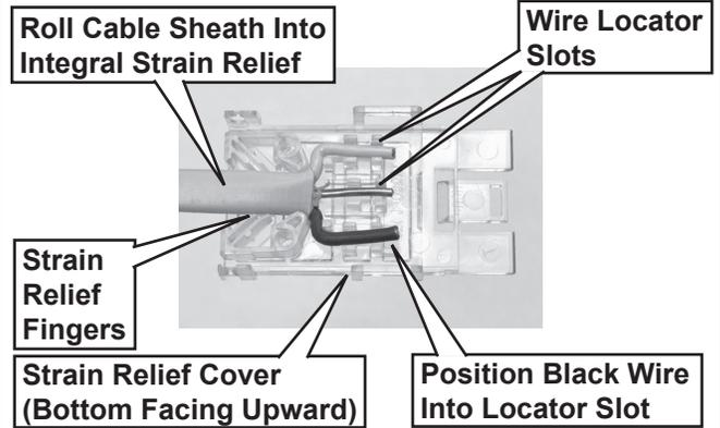
6. Lay wire into locator slots, making sure the black wire is placed into the polarization slot. See (FIG. 26).
