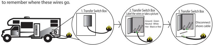
Step 3: Use the supplied male "plug/cord" in the kit and wire it into your transfer switch or main breaker.
