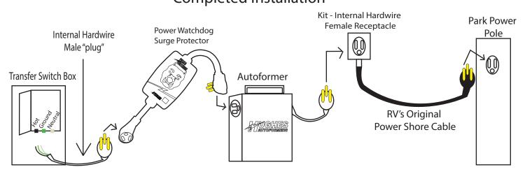
Note: If you are using an autoformer, it must be connected to the pole first before any EPO or EMS device.
