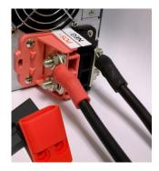
The WF-5118/WF-5120 inverters require 2/0 AWG input cables and a 250 Amp in-line fuse.
