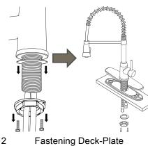
Apply plumbers putty or other suitable sealant to the bottom edges of the base-plate (optional). Once applied, align base-plate and press into place to firmly attach to sink. Remove excess plumber putty and place deck-plate onto base-plate. See images below. If installing on a onehole sink installing the deck-plate is optional.
