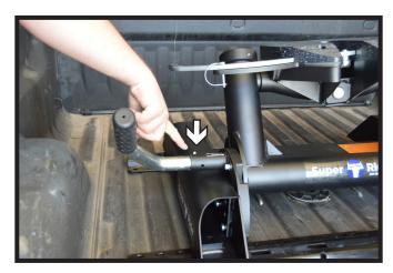
2. The handle is now locked into the grove on the side of the tubing.
