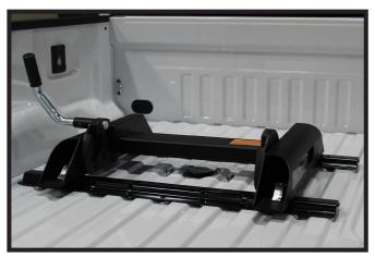
3. Set the hitch base onto the industry standard rails (ISR).
