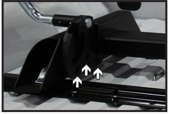
2. Recommended clearance between truck bed and 5th wheel trailer is 6-8 inches. To adjust the height of the Super Ride's hitch head remove the three (3) bolts holding the slider cam plate and adjust appropriately. Do this for both driver side and passenger side ensuring that both sides are equal in height.
