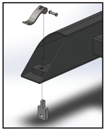
Customer will need to insert the ISR tabs into the base assembly. Tab is inserted from the bottom of the base assembly. Cam-lock is inserted into the top of the base and pinned to the ISR tab.
