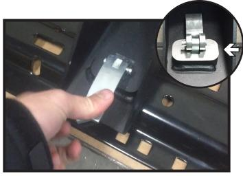
4. Close cam tabs to attach the hitch base to the rails.
