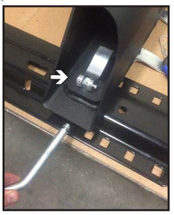
Make sure that all cam tabs are open and insert the four (4) 1/2" x 3" pins. Attach the clips to the back of the pins
