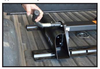
Release locking handle by pulling the handle towards the rear of the truck bed. Then pull the handle outwards and then towards the truck bed again.
