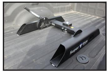
Release locking handle by pulling the handle towards the rear of the truck bed. Then pull the handle outwards and then towards the truck bed again.
