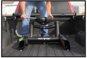
5. Set the hitch head on top of the shock towers.
