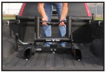
Center the shock towers over the hitch base vertically. Align the two (2) pins, one (1) on each side, with the grooves on each side of the hitch base and set into place.
