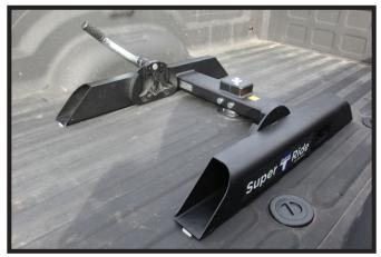
Place the base of the hitch onto the gooseneck 2-5/16" hitch ball.
