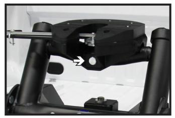
6. Insert the pin through the front of the hitch and then insert the clip on the back of the hitch to secure the hitch head to the shock towers.
