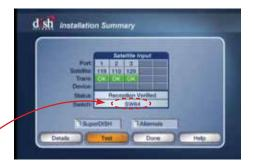
When you see the SW64 as the installed switch, the antenna is ready for use.
