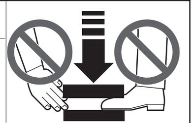
■ REMEMBER TO KEEP HANDS AND FEET OUT FROM UNDER THE FOOT PLATE WHEN USING THE POWER JACK!!
