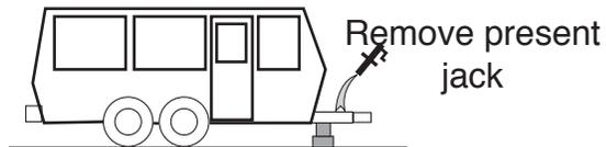
Raise your travel trailer's front end and place blocks or stabilizing jacks under the front "A" frame. Lower the trailer until it rests securely on stabilizing jacks or blocks. Retract present jack and remove.
