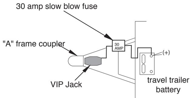
Connect the lead-wire directly to the positive (+) lead of the travel trailer's battery using a twelve (12) gage wire. Be sure the connection is a good one.
