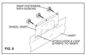
4. Take the 3 inch pieces of hook and loop strip; remove peel strip and stick them onto the screen room skirting opposite the hook and loop strips on the wheel cover. See FIG. 6.
