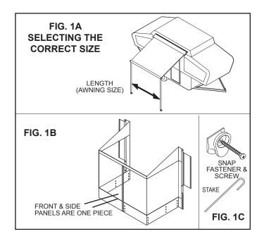
The above-mentioned panel and skirt are secured to the vehicle, the awning and to the ground by means of zippers, snap fasteners, PE clips, and hook stakes (provided). See FIG. 1C. **Note:** The inner and outer sides of all panels can be checked by looking at the snap fasteners. The round black plastic ring in the vertical edge hems is on the inside surface.
