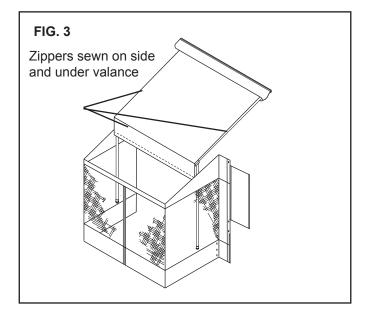
5. Fasten front of screen room to Trim Line bag awning by joining zippers. Start at awning front and fasten side panels to bottom side of awning. When attaching screen room to awning at bag, pull bag down and away from awning, making sure screen room is fastened completely.
