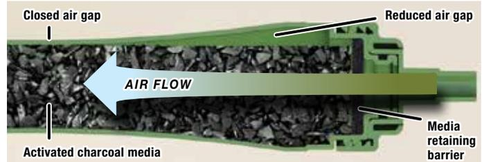
Charcoal media can settle inside a horizontal vent filter casing and leave a gap through which unfiltered air may flow. To reduce that possibility, SeaLand ECO is concave so that the settling media will completely fill the middle, forcing all malodorous gas to pass through the activated media for maximum odor adsorption.
