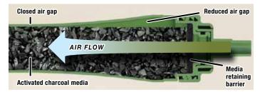
Charcoal media can settle inside a horizontal vent filter casing and leave a gap through which unfiltered air may flow. To reduce that possibility, SeaLand ECO is concave so that the settling media will completely fill the middle, forcing all malodorous gas to pass through the activated media for maximum odor adsorption.
