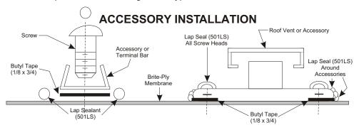
Caulk all screw heads, front and rear termination bar and all accessories. Note: Only Butyl Tape can be used with Brite-Ply membrane to assure proper seal.
