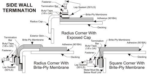
8. Apply butyl tape (BT-1834) to the termination molding. On the front, the front cap should lay on top of the membrane. Using a screw-type fastener, install the termination moldings - making sure there is sufficient roof structure. On the rear of the vehicle, the membrane should lay on top of the rear cap.
