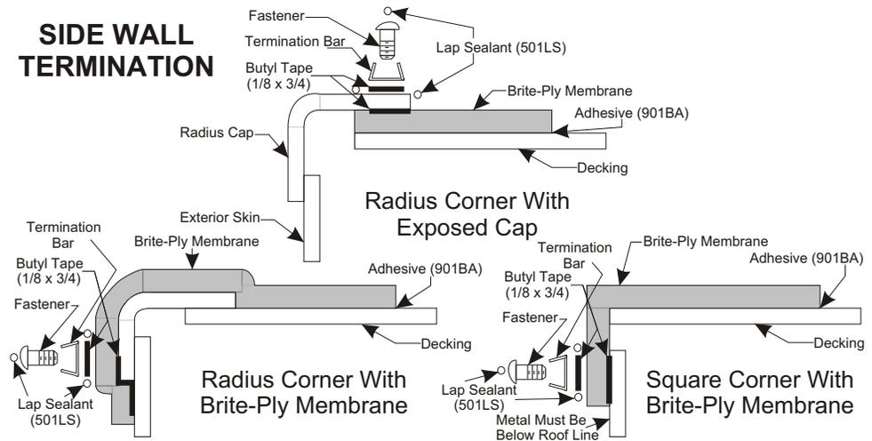
8. Apply butyl tape (BT-1834) to the termination molding. On the front, the front cap should lay on top of the membrane. Using a screw-type fastener, install the termination moldings - making sure there is sufficient roof structure. On the rear of the vehicle, the membrane should lay on top of the rear cap.
