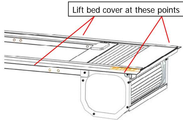
(NOTE: If needed, gently push and twist the rails slightly inward to drop into place. If there are aftermarket bed rail caps or an over the rail spray-in-liner installed, then the white nylon rail adjustment screws may have to be turned counter-clockwise 2-3 complete turns. Turn out **all screws evenly** until the cover drops into place.)
