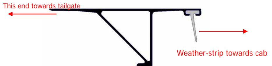
Front cover weather-strip must lay flat across the truck bed. If weather-strip extends past the rails, cut to fit right up to the rail bed capon the truck bed.
