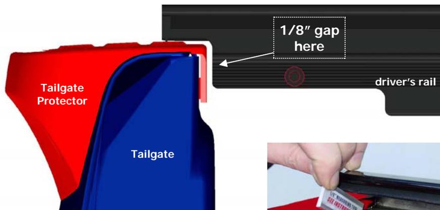
**Note:** Plastic bed liners may have to be cut at the front of bed so the bed cover can be moved forward to achieve proper 1/8" clearance at the tailgate.
