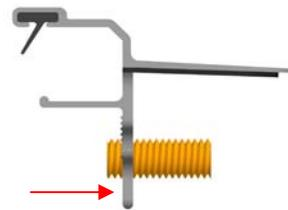
\*If the rails are too far apart, turn the adjustment screws in. (clockwise)
