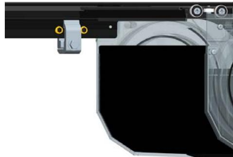
The clamps should be installed as high up as possible to engage more teeth on the rail. Using a 9/16" or 1/2" wrench, tighten the clamps. If the clamp wants to rotate while tightening, hold with pliers or vice-grip.
