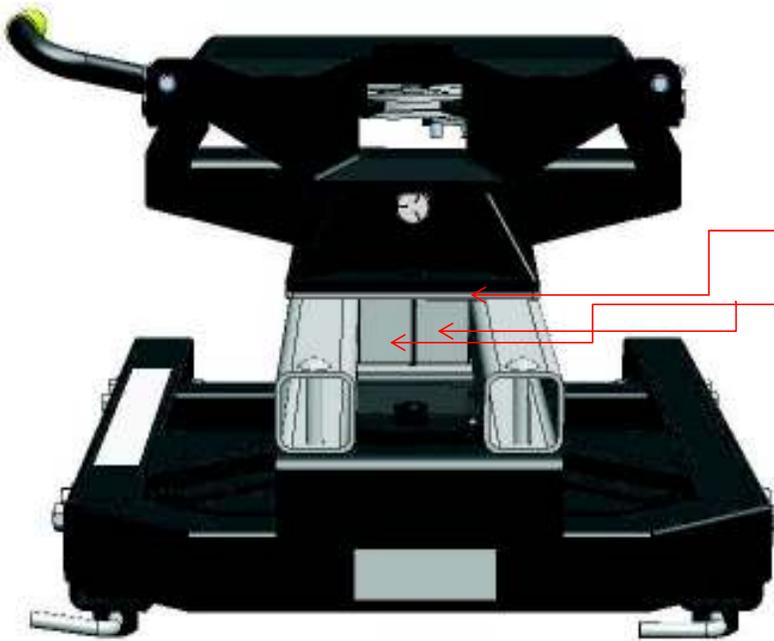
The 'Delrin' 'Wear Plate & Blocks' of the SuperGlide's Turntable Cam Arm Assembly were designed to glide along the surfaces of the 'Way Tubes' and around the Cam Arm's round shaft without the need for heavy lubrication.
