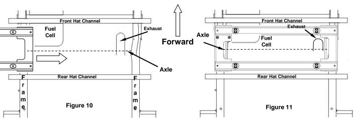
Step 1: Slide the base rail system in between the hat channels. Lift and position it so that it rests on the frame.
