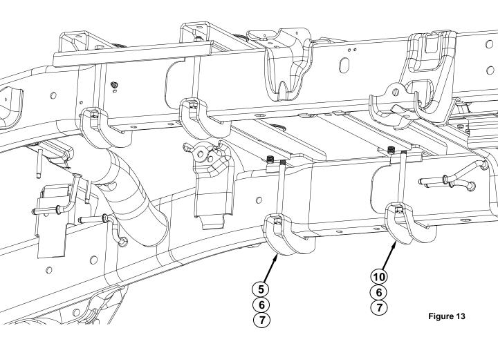
NOTE: Tighten both sides simultaneously to keep brackets even. The bolts (6) should be tightened to 75 ft-lbs.
