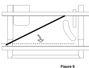
Step 2 : Continue rotating the rail up and over the exhaust so that it is against the rear hat channel
