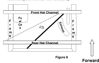
Step 1 : Slide the rear rail in at an angle over the axle and in front of the exhaust. Lift and rotate it so that it rests on the frame (drivers side)
