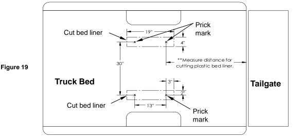
12. Remove 5/8" x 1 1/2" bolts attaching frame bracket to mounting rails. Move rails rearward or forward to prevent interference with hole drilling or punching of the truck bed.
