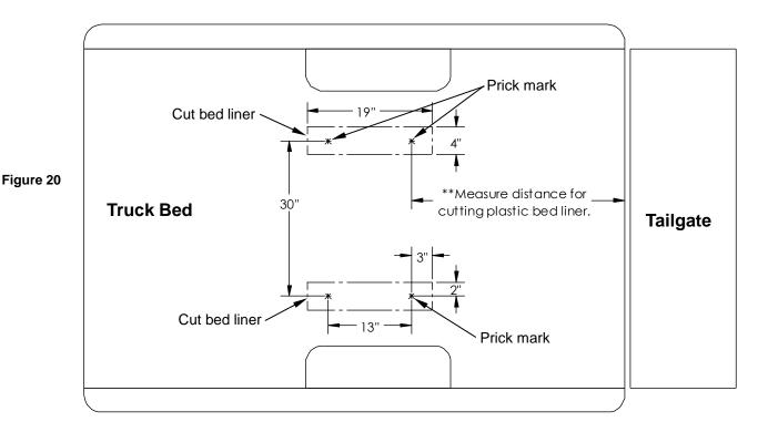
13. Move rails rearward or forward to prevent interference with hole drilling or punching of truck bed.
