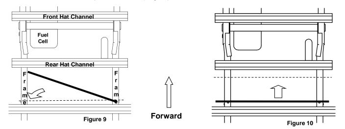
Step 1 : Slide the rear rail (shorter length) in at an angle over the axle. Lift and rotate it so that it rests on the frame (drivers side)
