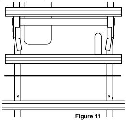
Step 3: The rail should now be near the rear hat channel with both ends resting evenly on the frame
