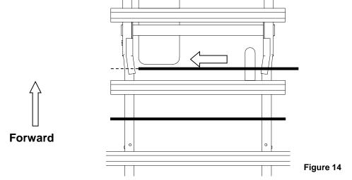
Step 6: Lift the free end of rail and slide the rail so that it rests evenly on both sides of the frame
