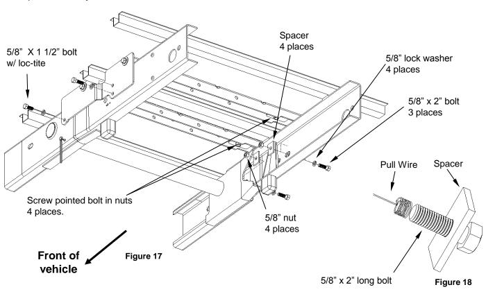
10. Using pointed bolt (**Figure 19**), screw pointed bolt in to the nuts that are welded to the rail assembly to make four prick marks. (**Figure 17**) If a plastic drop in bed liner is being used cut 19" X 4" slots in liner measured from prick marks in truck bed. (**Figure 20**) If the *Elite Series* slider fifth wheel assembly is used, then see fifth wheel slider assembly instructions for slot cut dimensions.
