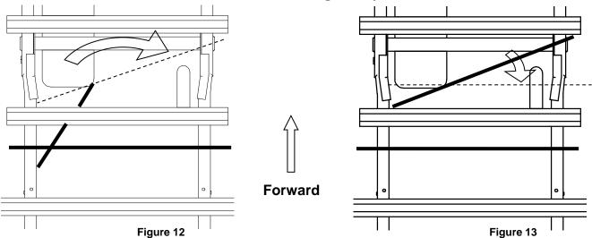
Step 4 : Slide the front rail (longer) in at an angle over the axle, over the exhaust and unto the frame (passenger side)
