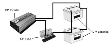
\*Installation using two 12 volt batteries.
