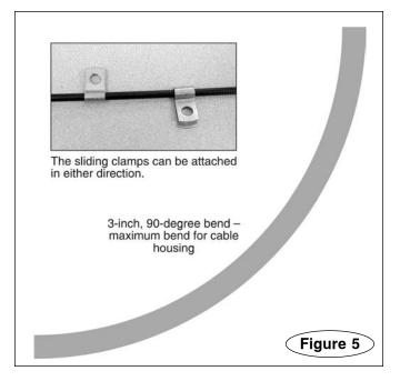
three-inch, 90-degree bend. Otherwise, InvisiBrake will not release braking pressure after it is activated, which will cause significant non-warranty damage to the towed vehicle's brakes and tires. Other consequential, non-warranty damage may also occur.
