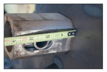
**2.** Adjust the top bolt so the top of the bushing measures approximatly 1/16" less than the measurement from the straight edge to pin. Pull the B&W pin and install adapter into the socket. Allow the B&W hitch pin to slide back into place. If pin in not fully going back into place, the adapter my need to be adjusted.
