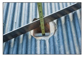
**1.** To install the adapter, lay a straight edge on top of the truck bed and measure from the straight edge to the top of cross pin.
