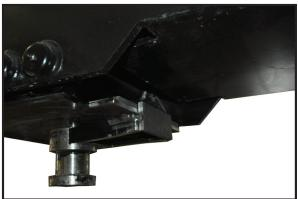
. Slide locking plate on back lip of Tri-Glide base. Center locking plate behind the king pin by pushing plate against base shoe. Clamp in place.
