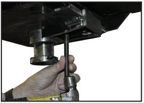
2. Using locking plate as a template, transfer/center punch hole location.
