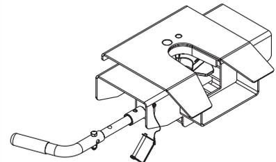
To uncouple, remove safety pin, pull handle straight out until the jaw locks open.
