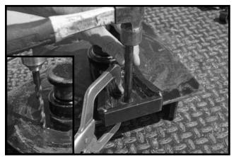
**3.** While using capture plate as template, center punch hole locations. Drill two 1/2" holes into glide ride base.
