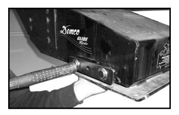
**5.** Inspect links and base for excessive wear and replace parts if needed. Lift kingpin base into pin box, lining links with holes in pin box. Install pin plates by tapping from side to side. Apply thread lock to end of bolt previously removed and fasten plate. Torque to 85 ft-lbs.
