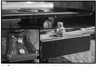
**4.** Fasten capture plate to glide ride base using the two 1/2" x 1-1/2" bolts and nylon lock nuts. Torque to 85 ft-lbs.
