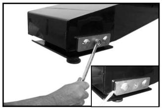
1. Remove 1/2" bolt from pin plate using 3/4" wrench or socket. Using a flat screw driver or thin chisel and hammer, tap between pin plate and Glide Ride box on bottom to get pin plate started coming out. Pry pin plate out by going from side to side by the 1" pin until pin plate can be totally removed. Be sure to support under kingpin base before removing pin plates. Lower kingpin base out of kingpin box.
