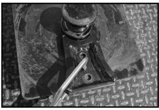
**2.** Center capture plate behind kingpin by pushing plate against base shoe. Clamp in place
