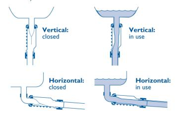
The Hep<sub>v</sub>O Sanitary Waste Valve opens under the water pressure of a fixture emptying and closes to form a tight seal after the fixture has discharged.
