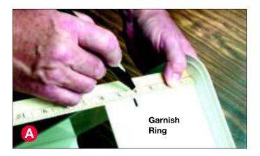
**7A** - After adding, in this example, 1/2 inch more, a line is drawn on the outside of the Garnish Ring at 4 inches.
