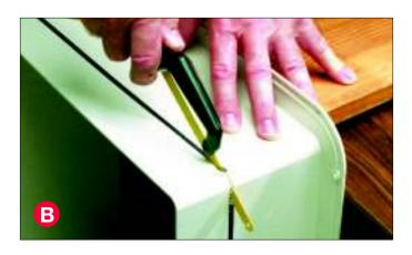
**7B** - Connect all four corners with a line at the required dimension and trim accordingly.
