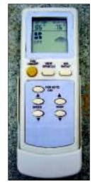
On Remote Control Models: Attach provided cradle to wall with (2) #6 screws provided. Handheld Remote Control may be placed into wall cradle for storage
