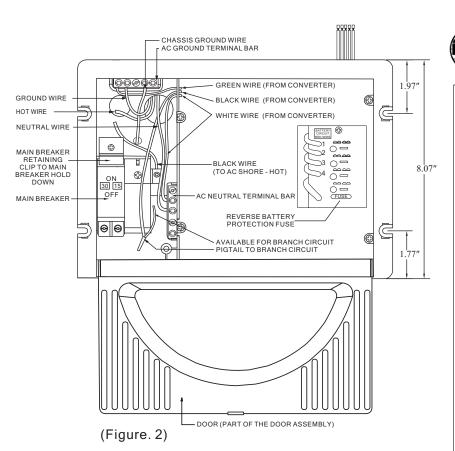
For proper wire sizes and torque requirements, refer to the label on the door assembly.
