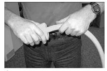
**2** Push cord through the inverted end about 18". A tug in the opposite direction returns boot to its original shape.
