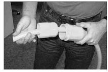
Push cord through plug/connector housing.
