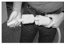
3 Push cord plug/connector housing. through
