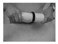
**8.** Lubricate mouth of weather resistant boot and rear shoulder of device with soap solution. Slide boot over the complete assembly. Be sure boot is on as far as it will go.
