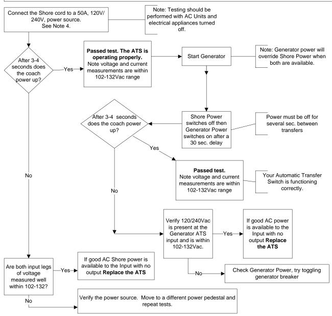
1. Line1, Line2 or Neutral open - Check all input wiring to the ATS. Check Shr cord. Check wiring on Generator. Replace Receptacle on pedestal. Replace adapter if reducing down to 120V,30A service.
